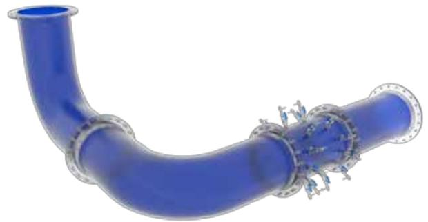
*flow meter after two out of plane changes in flow direction*
